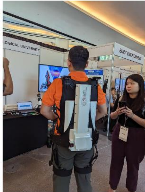
A back support exoskeleton developed by the National Robotics Programme. ST PHOTO: OSMOND CHIA
